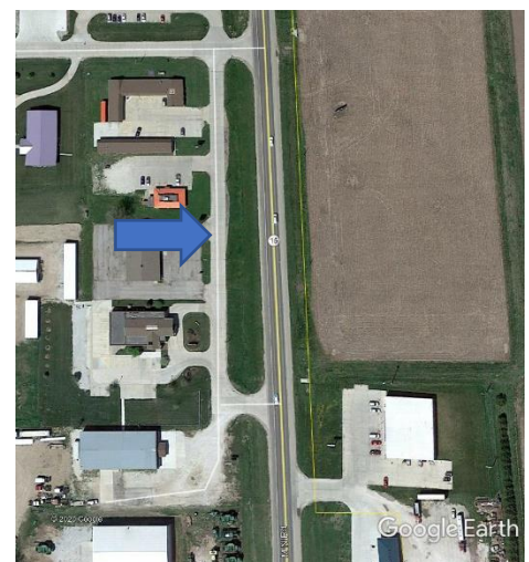
Example of a Frontage Road
